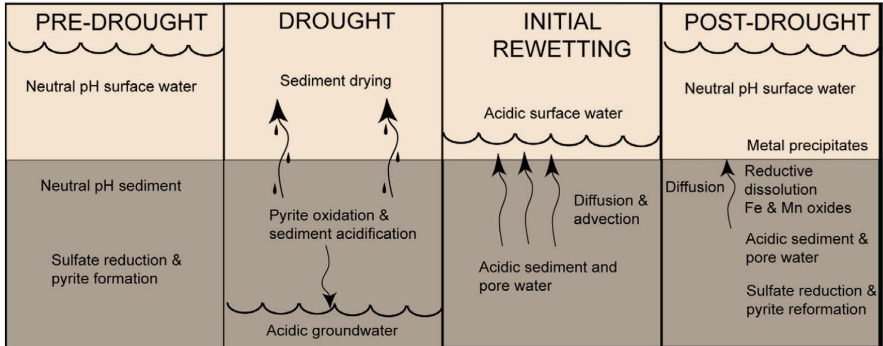
**Conceptual model of processes resulting in acidification of sediments and surface water during pre-drought, drought, initial rewetting, and post-drought conditions (Mosley *et al.* 2014)**
